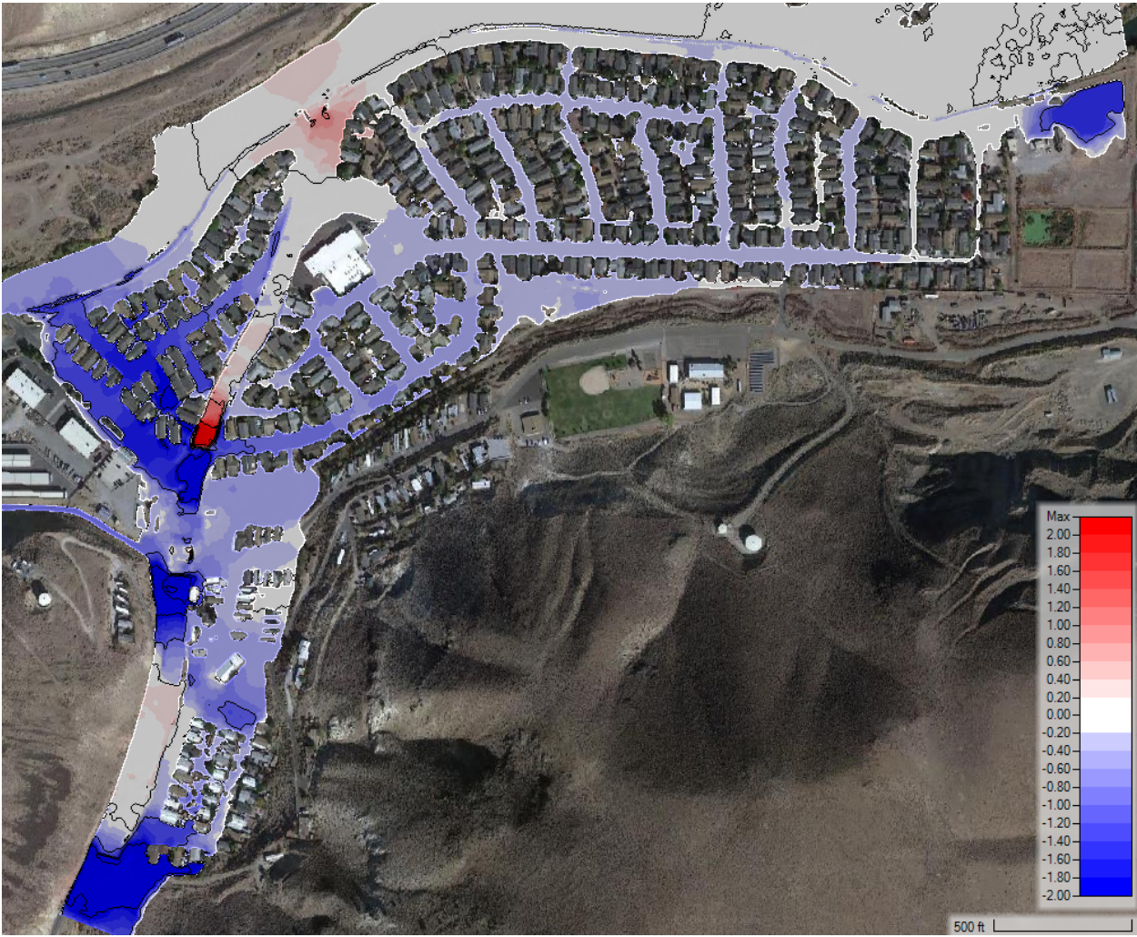
Figure 4-12- Comparison of peak water surface elevations for this alternative and existing conditions.
