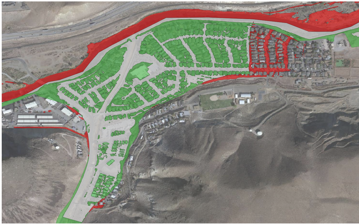
Figure 3-9 – Comparison of effective SFHAs for depths of 1' or greater and their modeled SFHA analogs.
